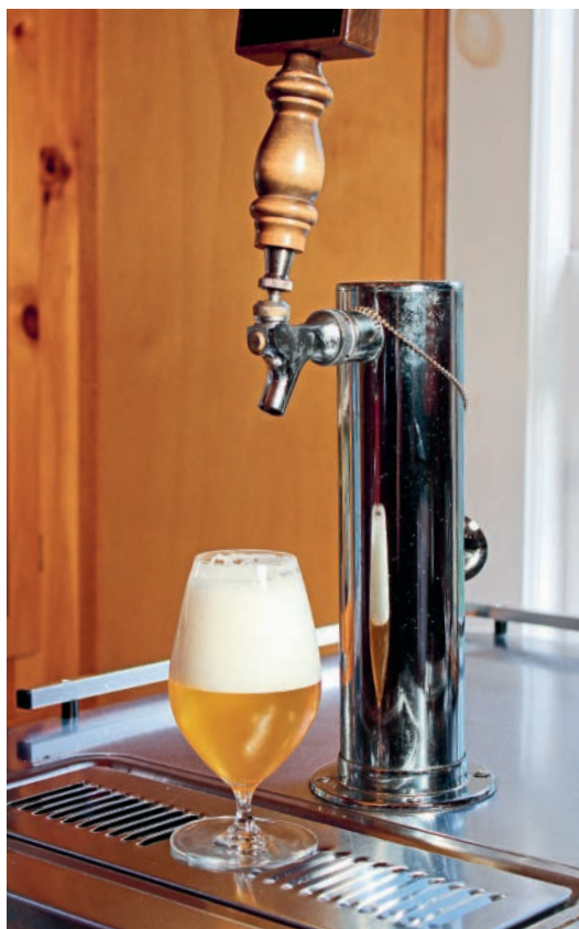
■ Foamy pours are a sure sign that your draft system is out of balance.
