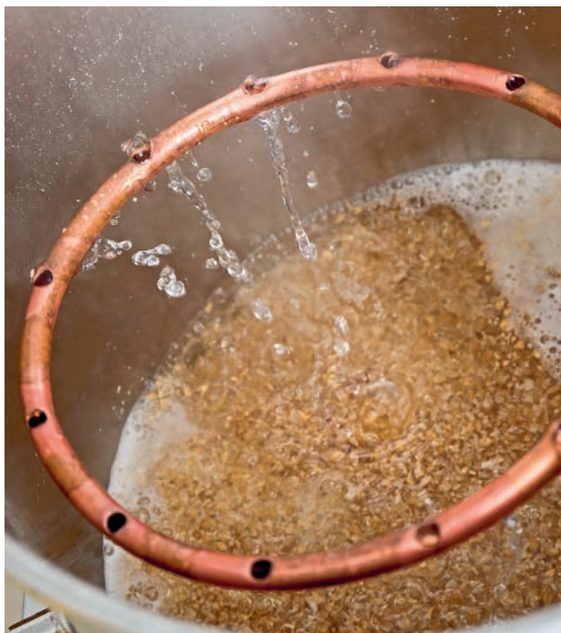
You can either batch sparge or fly sparge with a sparging device (shown here).
