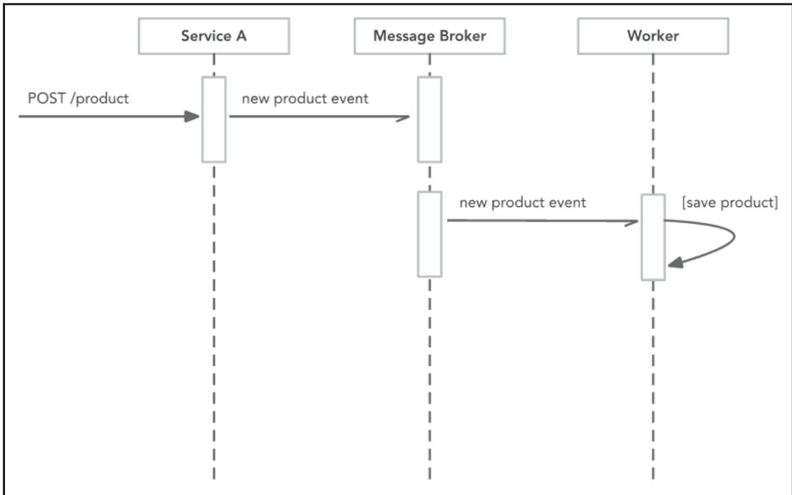
In this example, we are going to leverage the power of NATS.io to act as a message broker for our system, NATS is an incredibly lightweight application that is written in Go and provides such astounding performance and stability. Looking at `push/writer/main.go`, we can see that there is not very much code we need to write to implement NATS.io:
