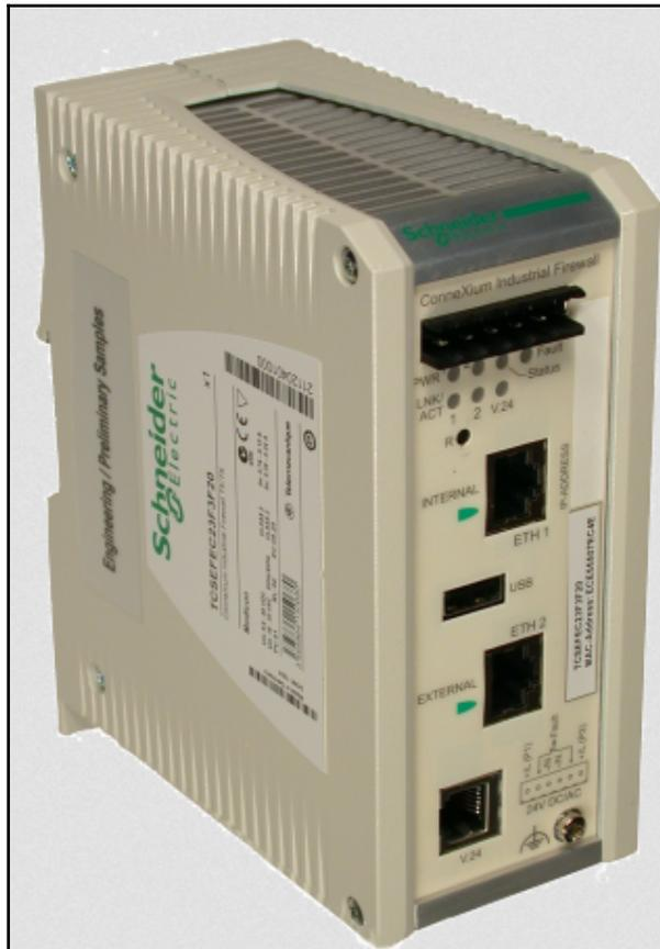
The Schneider ConneXium Tofino firewall
