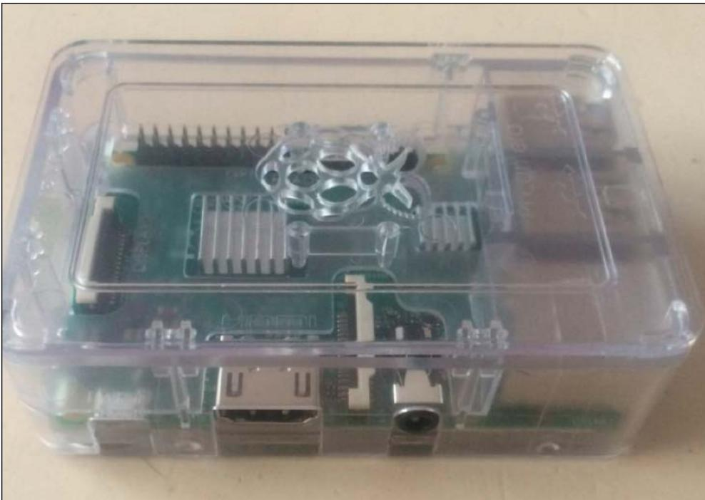
After that, the Raspberry Pi 3 was fully assembled, we merely hooked up our monitor via the **High-Definition Multimedia Interface (HDMI)** interface using the cable provided, which is plugged in our USB mouse and keyboard, and start preparing for the SD card for the operating system.
