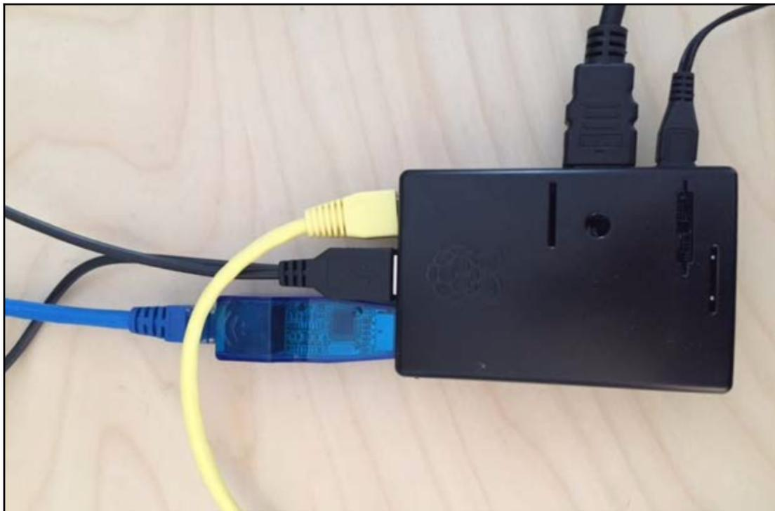
Now that we have the physical connection all set up, we need to configure our Raspberry Pi as a transparent bridge. In this situation, the Pi will be configured to have the same network or **Virtual Local Area Network (VLAN)** on both sides of the cables. This way, it can be inserted into a network segment between two hosts without any IP addressing changes.
