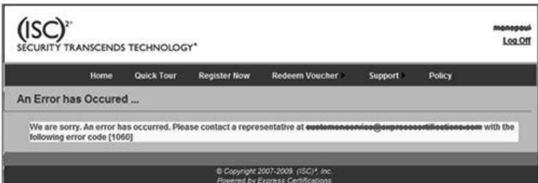
Figure 5.10 – Reference identifier used to abstract actual error details
